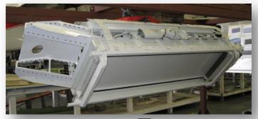
P-band high power amplifier in the nosecone (~15" x 22")
