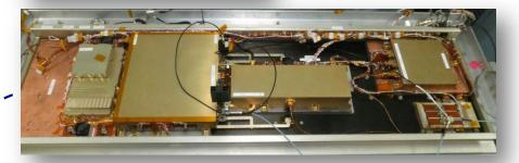
Ka-band high power amplifier and RF electronics are mounted to the backside of the antenna baseplate
