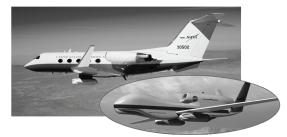
Originally developed to fly in a single pod underneath NASA's Gulfstream-III jet, the system has been modified to fly on the long-range high endurance Global Hawk UAV. UAVSAR's modular design is reconfigurable between multiple radar bands (L, P, Ka) and is used both as a flying test-bed for the development of future space missions and to gather valuable airborne data for ongoing Farth science research
